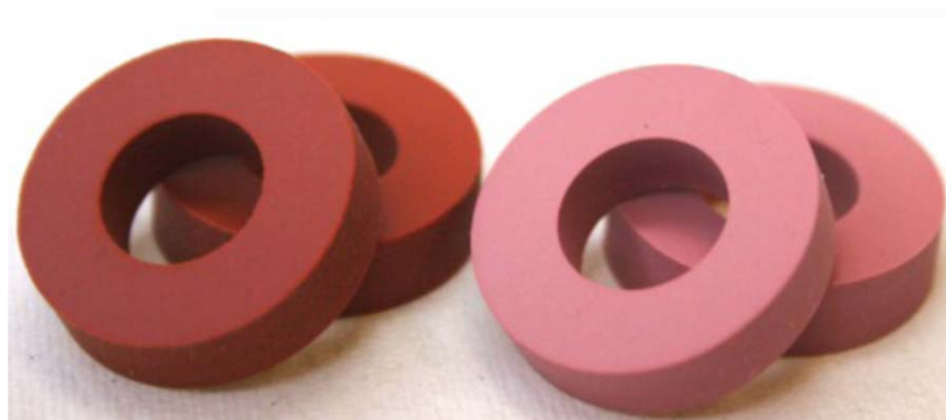
Figure 1. Small-scale seals: baseline on left, with 6% TiO 2 on right, 0.21 inches thick.
